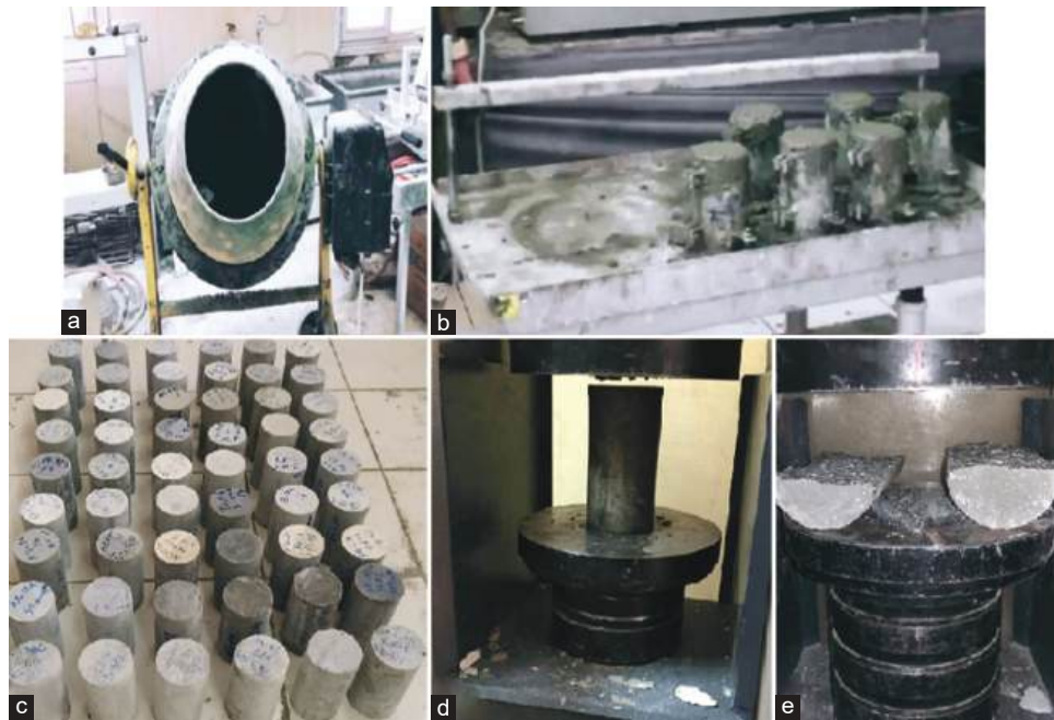
Fig. 4. (a) concrete mixer, (b) shaking table, (c) some of the cast samples, (d) compression testing, and (e) splitting tensile testing.
