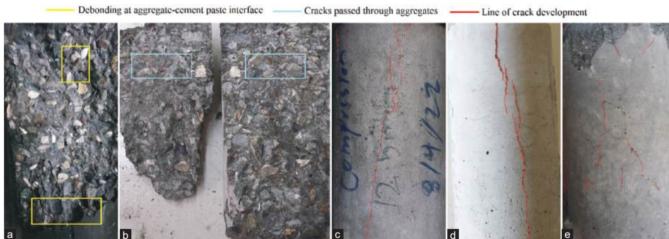
Fig. 7. Failure modes of tested concrete specimens: (a) Crushed gravel, (b) crushed limestone, (c) dolomitic limestone, (d) high-calcite limestone, and (e) natural gravel.
