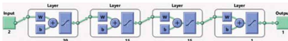
Fig. 10. Proposed neural network architecture of the designed low-pass filter with three hidden layers.
