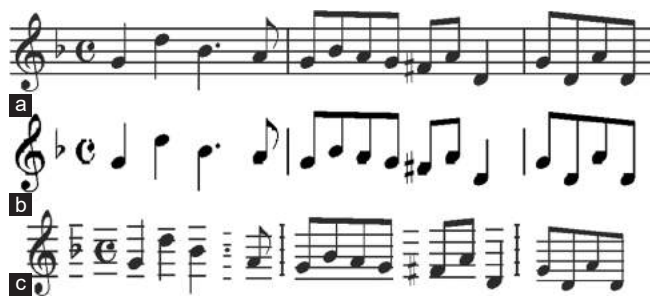
Fig. 2. Segmentation steps results, (a) the input image from (PrIMuS), (b) the image after applying the staff line removable function, and (c) the final segmented sub-images.
