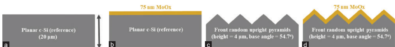
Fig. 1. Schematic diagram of ultrathin crystalline silicon (c-Si) (with 20 \mu m thickness) substrate (a) Planar ultrathin c-Si (without MoOx and upright pyramids) (b) MoOx AR layer on planar ultrathin c-Si; (c) front random upright pyramids (without MoOx) (d) front random upright pyramids with a front MoOx AR layer. The drawings are not to scale.
