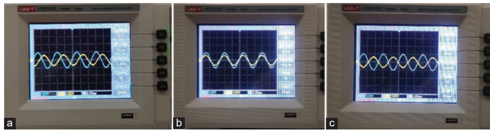
Fig. 11. Fourth order infinite impulse response low-pass filter (a) output of the filter, (b) phase angle between the input and output of the filter is 0°, and (c) phase angle between the input and output of the filter is 180°.
