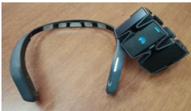
Fig. 3. Electroencephalography Muse four channels and electromyography Armband placement eight channels devices.
