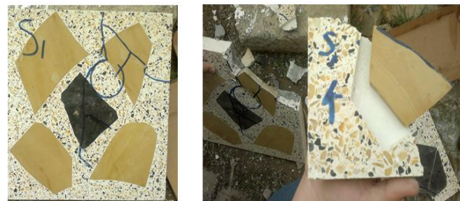
Fig. 10. Splitting failure of terrazzo tiles of factory (B).
