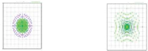
Spot diagram with effect of temperature Spot diagram without effect of temperature
